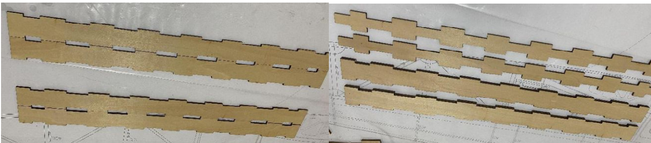
13) Glue scabbards, taking care to maintain the verticality of the scabbards.
