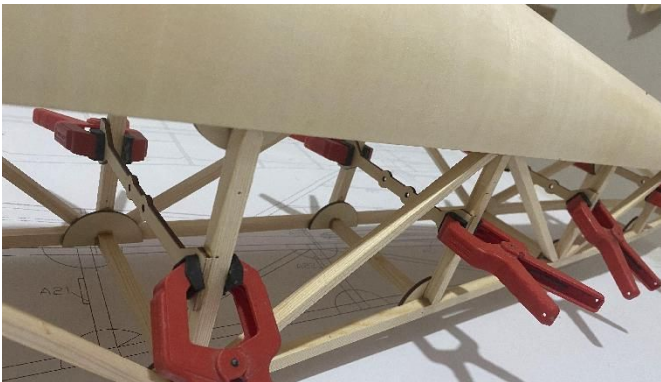
12) Glue pull-pull rods fixing seat.
