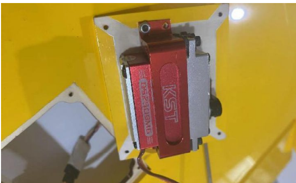
9) Fixing of aileron servos.
